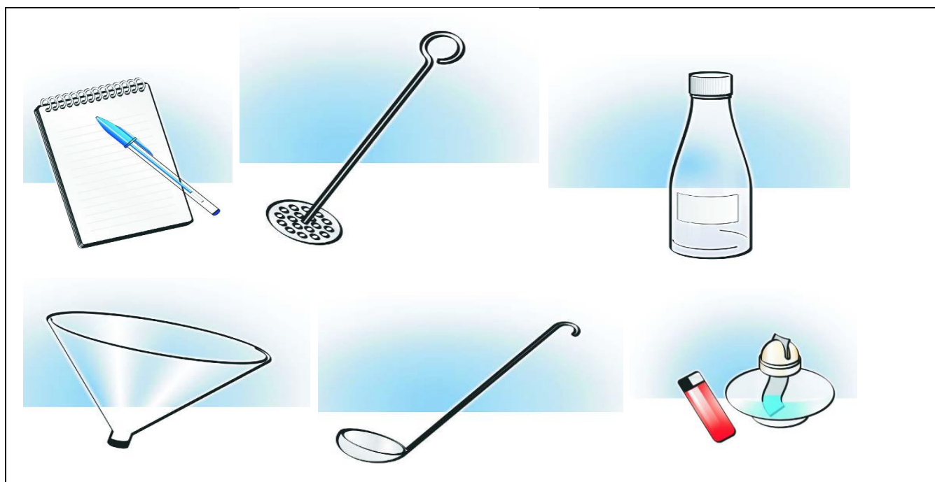
Figure 9. Milk sampling materials (Pen and note book, plunger, bottle, funnel, Dipper and sprint flame and lighter)
